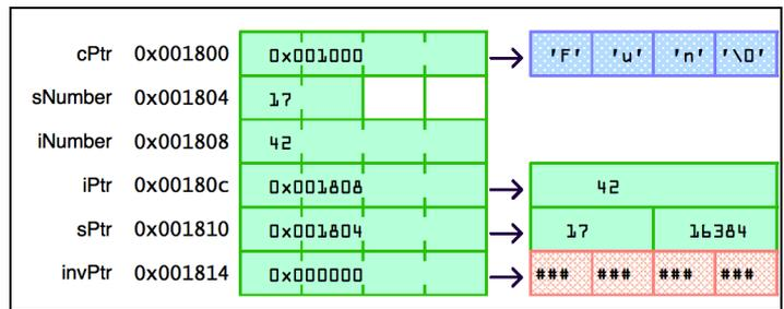
Fig. 1. Visualization of variables as memory blocks
